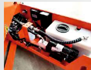
Bucher Elevating Hydraulic Pump Station
