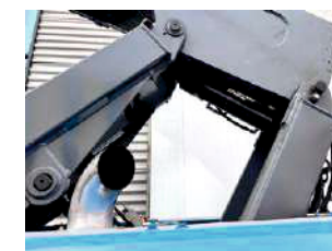
Lower Arm And Hydraulic Cylinder
