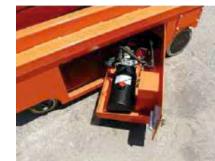
Hydraulic Pump Station and Motor
