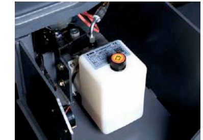
Hydraulic Pump Station
