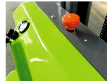
Emergency Stop & Indicator Light
